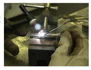
The stem of an ivy leaf doesn't really wrap around it's branch, I just did this for effect. Notice I am directing the heat behind the bend. This helps give you a very tight wrap.
