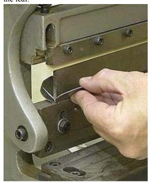
The leaf is pretty bent up, but that's a good thing. Notice how after I made a bend I had to bend the leaf back a bit to get the leaf in the press for the next bend. The unbending generates some waviness to the texture of the leaf.
