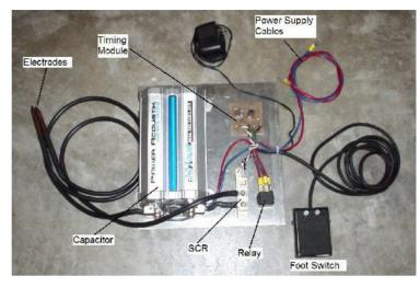
A foot switch triggered the timing module to disconnect the power supply from the capacitor. An electrical pulse was then sent to the SCR's gate. Release of the foot switch triggered relay closure, thereby recharging the capacitor. All this, of course, could be accomplished with manual switches.
