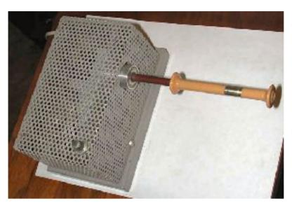
used. Bobbins come in two sizes. The photo on the left shows the smaller one. The long tapers were turned using both a tailstock center and the taper attachment on my old South Bend lathe. The spindles are held in place by a small O-ring and driven by a flat on their shafts. A small push button switch, located on top of the perforated metal housing, activates the winder's motor.
