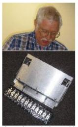
Dean Eicher (left) demonstrated an electrical test hook-up fixture that he made from aluminum sheet. It snaps onto a multicontact terminal block. By pushing spring loaded electrical pins against each screw connection on the block, electrical contact is established. A multi-wire cable transmits the signals from the contacts to an electrical test instrument.
