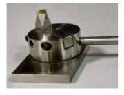
Martin Kennedy Demonstrated his internal and external lathe radius cutter. It uses two back–to-back triangular insert bits mounted at one end of a square slide. The device is normally affixed to a lathe's compound slide. The position of the bit relative to its pivot point determines weather it cuts an internal or external circular profile.
