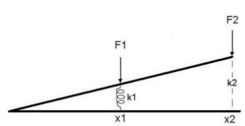
Now, an odd thing happens when you leverage a spring. The accompanying diagram shows a spring with constant k1 holding apart two arms of a levered hinge. The spring is located at a distance x1 from the hinge point. When a force F1 is applied at x1, the spring compresses vertically by an amount equal to (F1 / k1).
