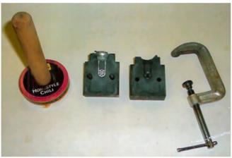
The left photo shows the die opened up, with the core pins that form a 1/16-inch square hole in the center of the handles to fit over a valve spindle. The diagonal scratches in the face of the mold blocks were scribed-in to vent any air trapped in the closed mold.
