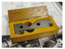
home made alignment tool for locating a horizontal milling cutter over a rod that would receive a centered slot (keyway) cut along its length.
