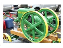
plant for a small Texas town for decades, ran 24x7 and they changed the oil while in service. Destined for the scrap heap, the Association has it on permanent display at their facilities, running it regularly. The announcer suggested we stand back, as starting is a diesel spitting process; huge black clouds of partially burnt fuel billowed skyward as the engine roared to life.
