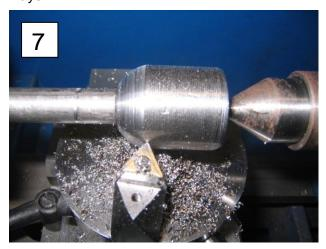
Now start making cuts on the right end (photo 8). I started with a piece that was a little too long, so I've got some excess metal to remove.
