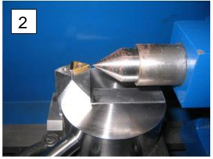
Photo 3 is a view looking down at the lathe. It shows the alignment of the triangular insert to the lathe's axis. Once you've set the on-axis adjustment using the cross slide, you should not move it again. If you do alter the lateral position, you might end up with an oblong ball. If possible, lock your cross slide gib now.
