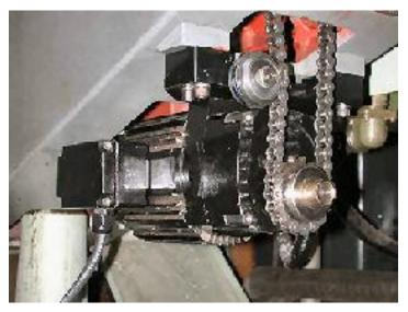
My mill, a Tree J-250, was purchased without a power drive for the knee. The mill has mounting pads for a motor that drives a sprocket on the actuating shaft up inside the knee body. The motorized knee option was discontinued before I purchased the mill. The parts manual shows a gear head motor with few details other than that it is a 0.5KW, 230 volt, three-phase motor, and that the drive chain is a ½-inch pitch chain with the dimensions in metric format.
