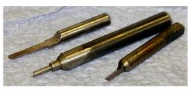
for a straight, V-pointed, non-spiral bit was introduced by D. G. Gordon. A detailed description of Gordon's technique for producing them can be found in <u>Live Steam Magazine</u> for August 1998, Vol. 21. Ed indicated that they are easily sharpened using his holder-jig along with a wet stone. It is nearly impossible to re-sharpen small diameter spiral bits (#60 and smaller) in the home shop.
