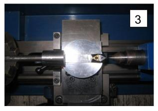
The stock is a short length of round bar that's been drilled, tapped, and mounted on a threaded rod that's held in the lathe's chuck (photo 4). Adjust the slider that holds the insert in the ball turner's head to a position so that it is just touching the stock. Then lock it down. It's OK to leave a small gap, since you'll be making the final cut after you move the slider in slightly. Note, I have not moved the cross slide, just the turner's slider.
