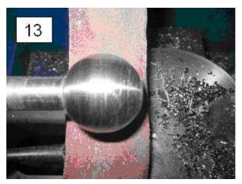
If you flip the insert over to the other side of the mount, you can use the ball turner to make concave cuts. Photo 14 shows the flared feet on shaft bearings that I made using this ball turner. Bon Ball Turning!
