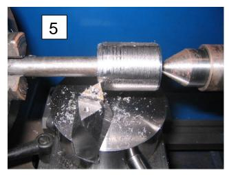
After each cut, I move the saddle very slightly to the right, and make a succession of cuts (photo 6). The stock looks like aluminum, but It's actually steel. You can, of course, use any material that you like. However, if you use an abrasive material such as phenolic, employ a vacuum cleaner nozzle to immediately collect the cuttings as they can damage the lathe's ways.
