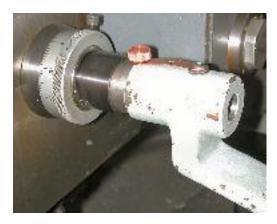
A spring-loaded plunger was fabricated and installed in the manual crank unit to engage an existing groove cut into the drive shaft. This prevents a spinning crank that could be dangerous (left photo). I recently fabricated a sheet metal chain guard, and the addition of limit switches is being considered.
