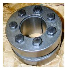
Bill Swann asked for suggestions on how to couple a drive shaft to the helical gear located at the output of an 3-phase electric motor. He and a friend are building an electric powered automobile. Presently, he plans to connect a drive shaft by clamping to the high points of the spiral gear teeth with the compression collet shown at the left.
