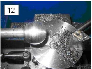
ball's surface. Remember to swing a little slower near the center of rotation, since the cutting speed is very slow there. When you're finished, use the cross slide to move the cutter away from the ball so you won't accidentally dig in to it, like I've done in photo 12.
