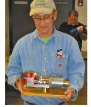
Randy Jacobs operated the Stirling engine that he recently designed and machined. He used a hand held propane flame for the heat source.
