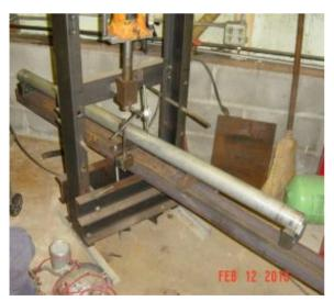
I placed a 6 foot long I-beam crosswise in my H-frame hydraulic press (left photo). V- blocks, located near the I-beam's ends, supported the tube. A long travel dial indicator, with magnetic base, was placed near the press ram so that I could measure the deflection as I applied pressure on the high side of the bend. The extreme resistance of the tubing to flexure surprised me.
