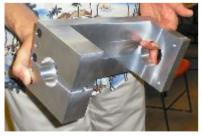
Lee Morin showed some of the parts he has designed and fabricated in order to convert a manual lathe to numerical control. He uses "Fortal" type aluminum and achieves the fine mirror-like finish with a variety of fly cutters that he passed around for member inspection.
