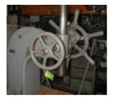
The arbor press that I recently refurbished is a Greenerd No. 3-1/2. It was missing the table plate, ratchet mechanism, and had a weld-repaired left side hand wheel. I replaced the original wheel with one from an old gate valve and revised the center bushing to fit the press pinion shaft. I added a heavy coil spring pressing against both a flat
