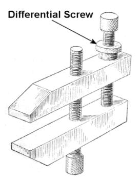
By placing a screw thread coaxially within another we create a differential screw mechanism. In the picture at the left, a long bolt passes through and threads into a bushing. The bushing has external threads that screw into the upper arm of the clamp. All threads are right handed.
