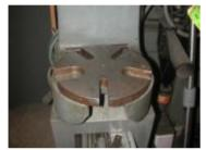
Next, I fabricated a steel table plate. The plate was turned from a section of flame cut mild steel and the slots were milled to look similar to the original. I used a 1-inch thick
