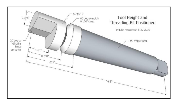
Using a dihedral hinge to gauge height and a V-notch to set bit alignment are certainly not a new concepts. What I've tried to do here is combine setting height and bit alignment into a single tool that slips into the tailstock ram's socket.
