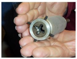
Dean Henning passed around a two-ended threading die holder (left photo). The holder is used in a lathe to assure thread alignment.
