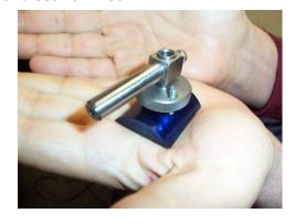
Chuck Rice brought in a headstock from a 1946 Atlas lathe that he was in the process of rebuilding (right photo). He also requested assistance on repairing a few broken pieces on the cast iron cover. Several suggestions were made – grinding and brazing using a fixture, epoxy, finding a replacement part on eBay, and making a new part.
