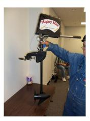
Gene Rowan showed his invention of a lightweight portable boat motor for short trips made from a trolling attachment powered by a cordless drill.
