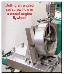
This 8 X 9 inch T-Slotted table tilts and locks in any position between 0 and 90 degrees. The T-Slots run both along and across the table's platen. It is machined entirely from mild steel plate and drill rod. Standard hardware fasteners are employed.
