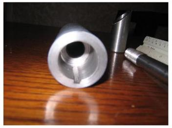
shaft towards the handwheel. Note that you have to make the shaft such that the larger section with the key slots is recessed in the body of the tool slightly so that it can move towards the handwheel. This causes the bottom section of the tool to offset at the 45° bevel, which wedges it inside of the spindle.
