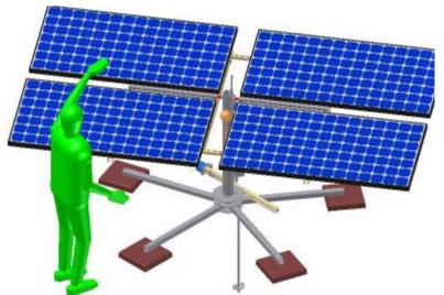
A second design, which he plans to build, tracks in two axes. It uses a stepper motor and worm gear for rotation azimuthally. A stepper motor turning a lead screw controls elevation.
