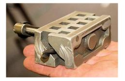
*Rich Pichler* challenged the membership to identify the purpose of a crude cast aluminum hammer he bought in Honduras. It turned out that it was used to crack lobsters.
