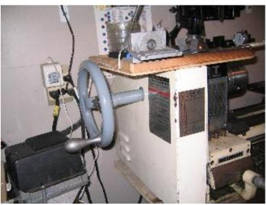
The ability to turn the chuck by hand solves this problem. By hand, you have excellent control of the stopping point and can easily thread up to a shoulder. I built a handwheel drive to let me accomplish this easily.
