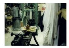
Rich's lathe is quite old, probably dating from the late 1800s or early 1900s. It does not have a nameplate, so it's unknown who originally made it. Rich bought it in early 1980 for \$125, which was a lot then. It was set up to be driven by a belt from an overhead line shaft. The ornate cast iron stand was drilled for a foot pedal adaptor. The lathe is a 10x20-inch. It came with two three jaw chucks and one faceplate.
