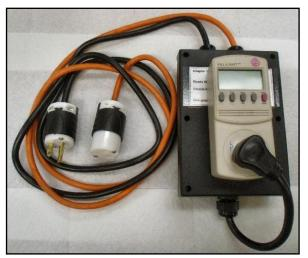
When the KILL A WATT meter is used with this 240 volt adapter, the indicated values of volts, watts, VA and KWH must be doubled. The remaining readings are just as indicated by the meter.
