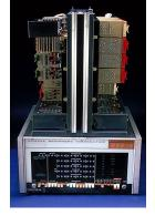
His next involvement with computers was with the first successful mini computer a DEC PDP-8 (left photo). This computer was available with 4-16k of memory. Input was with a teletype, and programs were saved on paper tape. It was the Swiss Army Knife of the industry and among other uses was employed to control mechanical processes. Dennis was involved in a project where a DEC computer was used to control injection molding machines.
