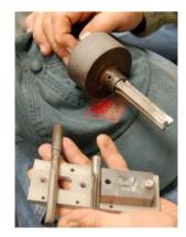
A Watts drill is one of several tools that can be used to create a square hole. You can use a square broach which makes sharp right angle corners but leaves partially rounded sides due to the oversize pilot hole. A Watts drill leaves slightly rounded corners with straight sides. A shallow square hole can also be made with a rotary broach, similar to the one Mike Winkler showed <u>last month</u>.
