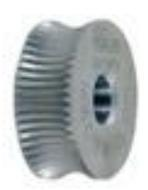
This project came to life when a friend wanted a small part rope knurled. A check of various catalogs indicated no source for such tooling. So, the next step was to make my own knurling wheel. I did not have a small tool to mill the wheel, so off to the lathe to start the process of making a special cutter after a little design
