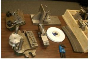
Side bends on the magazine holder were not straight, but were slightly curved to match the curved magazine. John made a die to make the 25.2-inch radius bend. It was necessary to over bend by 1.75 degrees to account for spring back.
