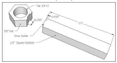
When you first screw your holder on to the Dremel spindle and bottom the thread against the motor's shoulder, you may find that the on/off switch and the spindle lock button on the motor's body are not facing upward. In my case, I needed an additional ¼ turn. Now, each full turn advances a 12-pitch thread by 0.083-inch. So, that extra ¼ turn of rotation required milling down the entire side of the holder by ¼ x 0.083 = 0.021-inch. I could have used shim washers to
