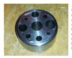
Martin Kennedy showed two things he made this month – a tapping alignment tool (left photo) and a milling vice speed handle (right photo). He described how he pressed in a deep socket for the hex hole in the speed handle.
