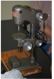
Chuck Rice acquired a Dunmore miniature precision drill from eBay. It had a pitted column and a bent spindle (photo left). He fixed it, straightened the spindle, replaced the chuck and painted it.
