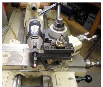
Here's a simple fixture that holds a Dremel motor in a lathe's Aloris style toolpost. It's fashioned from a reworked 5/8-inch hex nut that's silver soldered on to the end of a length of ½-inch square key stock.
