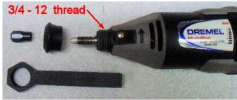
The 5/8-inch nut was bored and re-threaded as <sup>3</sup>/<sub>4</sub>-12 in order to fit the Dremel's spindle nose (above right photo). The over-all dimensions of a common 5/8-inch
