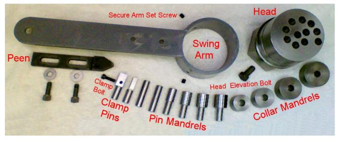
internal threads to 3.75 inch ID will yield just the right sized material for the collar. The swing arm's handle was brazed to the head collar. After brazing, I smoothed the handle's curve with a vertical oscillating drum sander to match the inside radius of the head collar. A rat tail file would serve as well here.
