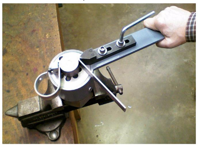
This radial bender can form arcs in both wire and flat stock up to 1/8-inch thick. Additionally, it will bend \(^1\)4-inch material that is heated dull red hot. It accommodates material up to 1-inch high with inside bend radii between 1/4 and 1-inch by using 9 round mandrels. I first saw this style of radial bender in a 1968 Popular Mechanics article in the Do It Yourself Encyclopedia, page 257.
