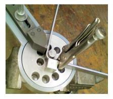
Thick work tends to pull out from under the clamp pin. This can be prevented by firmly grabbing the material being bent with a Vise Grip on the side opposite from where the bend is being performed (left photo). Alternatively, just tighten the clamp screw in the clamp pin (photo 2 below).
