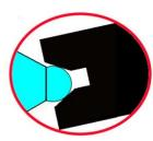
If you use a tool post grinder on taper turned work, ball tipped centers are essential in order to obtain a perfect circular grind (left drawing). The miss fit of the conventional 60-degree centers and the work's counterbored sockets will not provide maximum stability during the grind.
