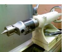
Now on a complementary note: Offsetting the tail stock may be easily accomplished, however, returning it to the lathe's center, when you've finished turning, can be challenging. Instead, use a mill's boring head to provide the set-over. Make a ball tipped center that fits into the head's straight shank boring bar hole and use the head's set-over adjusting screw to
