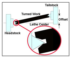
range of diameters, consider making several ball tipped centers having balls commensurate with the size of the center drills used.
