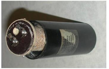
The capacitor in the photo was one of a pair that was from the motor on my air compressor. I recently noticed slow starting of the compressor, so I decided to physically check the capacitors. First I had to move the motor starter enclosure to gain access to the housing covering the capacitors. To my surprise, both capacitors had *blown their top*. The motor saw many years service on my lathe before being moved to the air compressor. It is a Baldor 3 HP motor that is now 30 years old.
