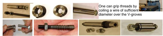
of the threads on a bolt, so that the thread crests are protected. A round bar with a tapped hole and slits on its side provides a clamping fixture for bolts when placed in a lathe chuck. A square or hex bar with internal threads and side slits provides a fixture to hold a bolt in a mill vice. Round collets will distribute the chucking force over the threads of a fastener being worked in a lathe..
