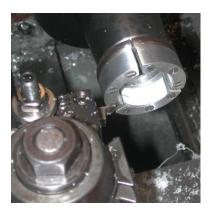
The photo shows a special modified collet that I made many years ago to cut off 11/2-inch OD acrylic tube into one inch long lengths. The stock is cut to length and then with a special radius tool, the ends are rounded over.
