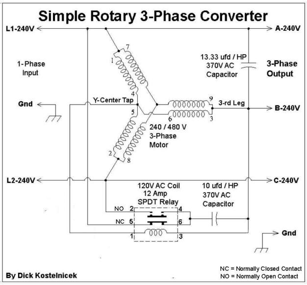
My converter uses a 7.5 HP, 1725 RPM, 240/480V, Y-connected, 3-phase motor. It is hooked-up with the electrical windings connected in parallel to accommodate 240V. Either a 1725 or 3750 RPM motor would work equally well. The only difference: a 1725 RPM motor will be a bit larger, more costly, and heavier in weight. I also sawed off the motor's shaft to prevent my tripping over it.
