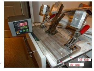
with a small aluminum plate. I put a piece of plastic bag both below and above the belt 's joint to keep the adhesive from sticking to the aluminum plates.
