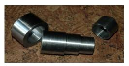
I tried to hold rings in a recess cut in an emergency collet but the rings had too much flex to seat solidly. When I tightened it up, they would bulge out in places. So, I made an expandable arbor for machining the width (or height.) It has a 20 degree wedge which releases easily. Note the 1/8-inch
