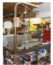
A member showed photos of a large hydraulically operated mill used to make parts for robots. Also, he showed a picture of a hoist that he made from 1 ½-inch roll cage tubing. (Photo left.)
