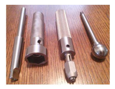
From the left, there's a ½-inch shaft made with an integral #2 Morse taper that fits directly into the lathe tailstock. My original kit had a rod that I put into a chuck that fits into the tailstock. Either will work.
