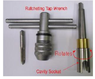
larger Morse taper, I can use the cavity socket to support tapping in a larger lathe.
