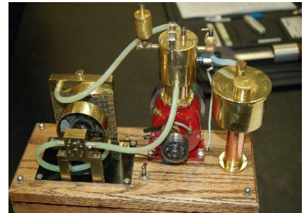
Alan May demonstrated the operation of a 1906 era four cycle engine. The engine uses acetone for fuel and has a 1-inch bore and 1-¼-inch stroke. Alan made the engine from plans designed by Jerry E. Howell (right photo).
