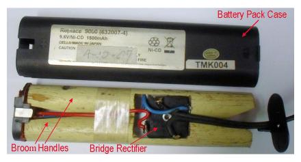
I have one of the early Makita miniature battery operated circular saws. The Makita brand 9.6 volt battery, which powered both the saw and a companion cordless drill, now costs around \$80. So, I moved on to other sawing options. However, I really love that saw with its 3.25 inch diameter carbide tipped blade. It performs well on wood paneling and acrylic sheets. It will even sever a wood 2x4, although you have to make a cut on both sides in order to completely cut
