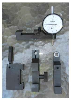
This new design makes changing the orientation of the dial indicator holder *tool-less*.
