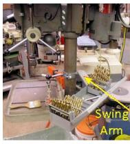
back in its proper spot in the drill case. Well there is nothing new here except that I vowed to change my sloppy ways by employing a swing out drill case.
