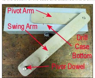
dowel pin. However, a loose fitting bolt with a lock nut would serve as well. (See left photo). The pivot arm then attaches to either the lathe bed or the drill press column (right photos) with an appropriate clamping fixture.
