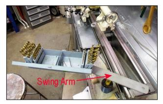
At the lathe or drill press, I use a variety of jobber sized drills. I had to walk over to my work bench, where I stored the drills, in order to get a particular drill from its case. After use, I often laid it down somewhere (not remembered later) rather than putting it
