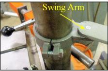
Now, I can stand at the lathe or drill press and select my drill bit. After use, I immediately put it back in the drill case without taking a step away from the machine. No more hunting for drills that were laid down at a convenient but forgotten place because I was too lazy to walk over to its drill case.
