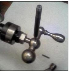
difficulty, I was able remove the stuck pin by pressing it out with a pin punch from the other side of the ball handle (right photo). The extracted pin was mangled and the holes in the lead-screw shaft and ball handle were both galled. So what went wrong?
