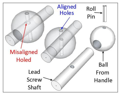
rotational orientation where the handle's ball and shaft holes were aligned. The roll pin was then pressed with ease into the assembly.
