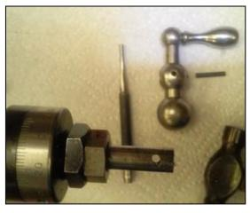
With ease I removed a ball handle from a lathe cross slide's lead-screw by pressing out the 1/8-inch roll pin with a pin punch (left photo).
