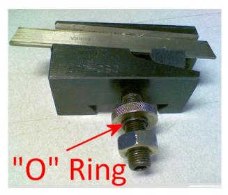
To roughly monitor the depth that a drill has penetrated its hole, I place an O-ring on the bit (right photo). I used to use masking tape for this purpose. This technique is useful on the lathe and especially when using a hand held drill motor.
