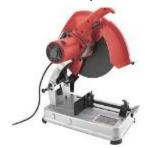
about \$10 to \$20. About 20 to 30 chisels can be made from one spring which often has multiple leafs. The leafs can be cut up with an abrasive metal cutting blade in a hand power saw guide (Right photo) or with a abrasive chop saw (Left photo). Make the chisels long enough to avoid hitting your hand (8-10 inches).
