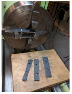
Or, you can do it the inexpensive way! I use milling parallels on my lathe. I have the type with holes in
