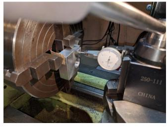
the chuck is mounted on the lathe, you can move it around with very small adjustments so that the parts don't fall out. You may also want to put something like a piece of cardboard on the ways underneath the chuck so that if (or when) your parallels fall out they don't get damaged.
