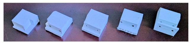
After the test installation of the first print, I found that the switch didn't actuate because it needed to be about 0.030" closer to the part the switch was to contact at the limit. I also had to move the switch about 0.050" farther away from the mill. I printed the second version, and continued to tweak the
