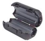
I solved this problem in two steps. First, I placed a 100 microfarad capacitor across the 12V power supply at the electrical input to the LED lamp. Second, I placed a clamp-on ferrite filter core (Left photo) using several wraps of both the 12 Volt power and Hall sensor lines going to the RPM indicator.
