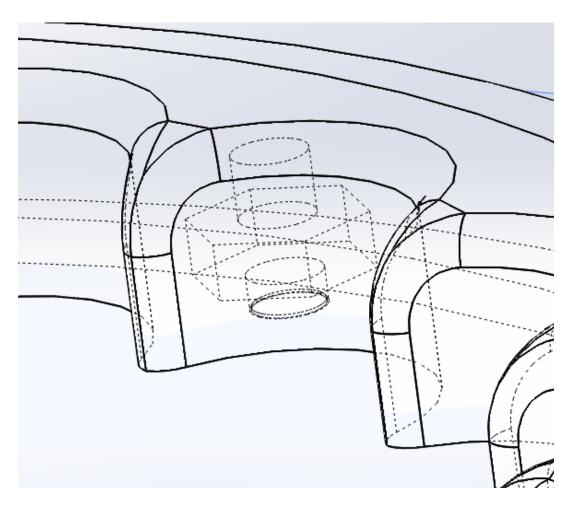
I made the hex cutout slightly larger than the nut because I wanted the nut to drop in easily. I made the cutout 0.015" wider than the nut, and 0.020" deeper. I'm using Repetier Host with the Cura slicer. I've also used Slic3r, but one of the features of Cura makes this easier.
