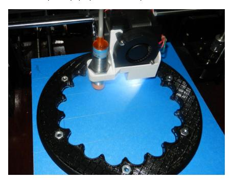
When your print finishes, you'll have embedded nuts! This same technique can be used to print layers in different colors. When the print is paused, change out the filament to the desired color and restart.
