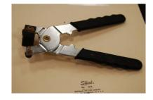
Brian Alley showed an alignment tool he designed and made for adjusting the axle on a motorcycle. See right photo.
