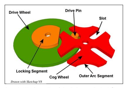
A Geneva Mechanism is made from two meshed wheels called the drive and cog (left illustration). The red colored cog provides intermittent, non uniform, rotary motion when the green colored drive wheel turns at a uniform speed. Click here to animate the motion.
