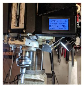
The maximum current that I expected for my 2 HP motor was about 6 amps. The nameplate on the motor said 5.5 amps, but I planned to measure the split-phase voltage upstream of the VFD, and I was not sure how going through the VFD would affect this. I had observed about 6 amps on the ammeter I had, so I was fairly confident that a 20 amp range on the PZEM-021 would be adequate.
