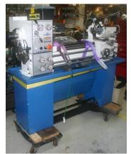
end required me to use a pry bar/scraper to wedge up the lathe and was finally able to remove it by lifting with the engine hoist. Removing the last of the caulk was difficult as the caulk removers also removed the paint.
