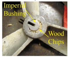
straight imperial key bushings. I selected a bushing whose diameter just cleared the small end of the tapered pulley hole and had a slot for a 3/16-inch key. This key slot is 0.1875 as compared to 0.1968 for the wider 5 mm woodruff key. I forced the slotted side of the bushing against the hole's taper with hardwood chips (left photo) and broached the hole.
