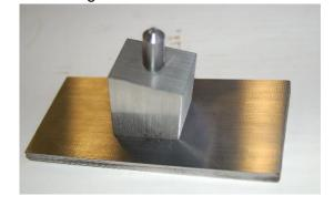
Also, John showed a grinding wheel dresser tool he made for truing a grinding wheel. See photo at right.
