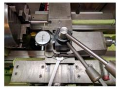
If the stroke of the compound is not long enough, you'll need to release and reset the saddle lock and move the saddle further along the taper. Cut until it blends in to the original cuts.
