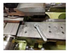
First LOCK THE SADDLE! You will be making this taper by moving the cutting tool using only the compound, not the carriage. Accidentally moving the carriage will ruin your part.
