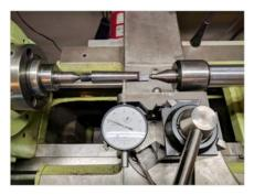
Mount the reference taper between centers. Centers are required, as we'll be moving the tailstock away from the centerline, and when making cuts, the stock will wobble in relation to the live or dead centers.
