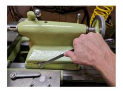
When you finish making the copy, you'll need to reset the tailstock using a tailstock alignment bar. If you don't have a bar, here's another method.
