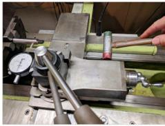
Measure the large end of the taper, and cut until it matches specifications. Note that Machinery's Handbook gives a diameter that's not at the end, but a little back. I measure the diameter at the end of the reference taper, and cut until I hit that.
