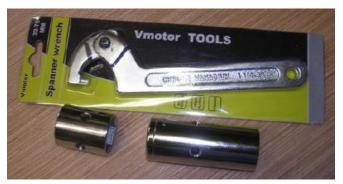
Use with either a standard or deep socket. You can use a spanner wrench or make a handle as shown in the previous version. (left photo)
