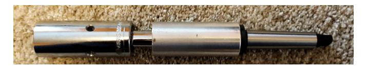
Sleeve used to position the die in the socket. (right photos)
