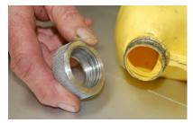
John Hoff displayed a cap he made to fit a plastic container to facilitate the flushing of the a/c compressor of his car. See left photo.
