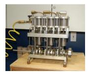
steam successively expanded in two cylinders on the same shaft. Later, as technology of the time advanced, the introduction of three compound cylinders on a common crank shaft represented an improvement over tandem cylinders. Some of the problems with single and tandem cylinder engines were making them reversible and capable of starting from dead stop at any point in their revolution. The Stephenson Engineering Co. developed a valve gear mechanism to make multi cylinder engines reversible.
