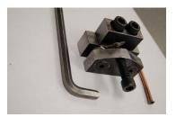
John Hoff exhibited a flaring tool he made to shape steel brake lines on a vintage car he is restoring. (See left photo.)
