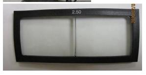
Brian Alley displayed a set of welding helmet magnifier lens (aka cheater lens) he purchased recently. Unique about the lens is that they are made of glass. See photo at left.
