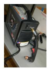
Major parts of a plasma cutting system include a power supply, torch, and a gas supply.
