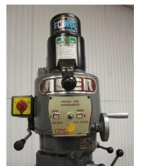
Joe Sybille exhibited a key made on a mill with a pneumatically operated drawbar. He found using the drawbar convenient, as there was no need for a wrench to loosen or tighten the drawbar to remove or install the spring collet holding the end mill. See photos at left and right.
