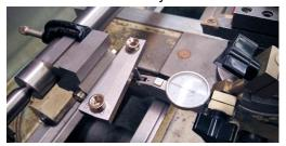
The lathe's compound angle was set to 8 degrees by traversing a dial indicator along the angle block. When the reading held constant, the angle setting was achieved (see left photo).
