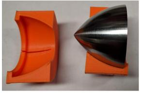
To hold the part, I made a fixture on my 3D printer. It exactly fit the outside of the shape. I had cut the Reuleaux shape using CNC, so I already had a CAD model of the puzzle. This made it fairly easy to design the mating 3D part.
