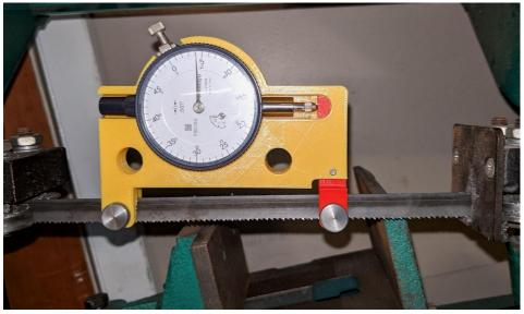
Here is an update on my August 2011 HMSC article Setting Tension in a Band Saw Blade (see page 7). When I wrote it, I designed a gauge that would help in the measurement of the tension. The article had a lot of detail on calculating the desired blade stretch. The article concluded with me deciding to not build the gauge. Instead, I used a caliper to measure the stretch.
