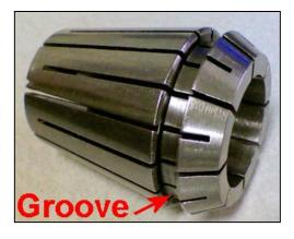
ER collets have an external retaining groove (left photo) that snaps into a circular clip (right photo) built into the collet nut. That clip is offset to one side of the nut's center. A difficulty results when inserting the groove into the clip. Simply pushing
