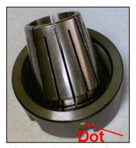
Here is how to make the collet engage and disengage the nut. Tilt the collet relative to the nut's circular axis (left photo). Insert the collet grove into the nut's offset clip. Then, rotate the collet axis back to that of the nut. In order to locate where to tilt the collet relative to the nut, put a shallow hole ground with a carbide ball bur and filled with a **Dot** of white paint on the outside
