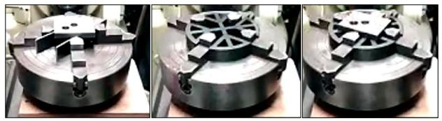
When using a self centering chuck one should always use a dial indicator to ascertain if the workpiece is actually centered. Sometimes a tap on the workpiece with a small hammer will aid in centering. The addition of a shim between the workpiece and the chuck jaws helps with centering. Kennedy uses the thin metal from merchandise security strips for shims. These metal strips are about 0.001" thick and come free with some items purchased at stores.
