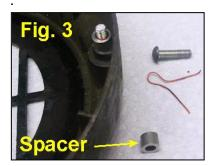
So, here is my solution and it should be good for the rest of my lifetime. Since I couldn't move the fan closer to the motor body, I moved the shroud away from the warped fan blade by ¼ inch with spacers (Fig. 3). Now you need more than 2 hands to secure the shroud to the motor with spacers on its 3 mounting screws. And all this is to be done in the prone position with head inside an
