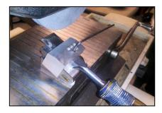
Dick Kostelnicek exhibited a fixture used with a surface grinder for sharpening chisels and other items requiring a sharp edge. See photo at left.
