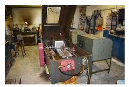
At the left is the 24 inch hydraulic feed saw. Its advantage is it puts a constant pressure on the blade and therefore cuts much faster.
