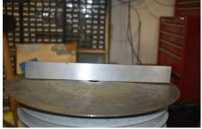
Shown at the left is the smaller blade after I put it in the press. The dome shape was much worse before.
