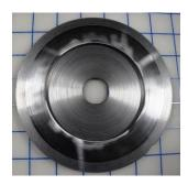
John Cooper showed a flange he made for a 24 inch diameter rock saw blade. The flange is made from 3/8" thick steel plate (left photo). Also, he showed a Cleco rivet fastener. Cleco rivets can be installed where there is no access to the opposite side of a workpiece (right photo).
