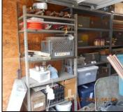
On some of the shelving units the bottom 3 feet to 4 feet is devoid of flat shelves. This allows the storage of movable tools on wheels to fit within the shelving unit proper. Some shelving had fabricated pull-out shelves. This facilitated retrieving items placed at the back of the shelf. Reinforcement steel shapes of at least 1"x1"x1/8" were added for extra support as required for heavy equipment or wide shelving.
