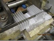
Shown at left below are the two heatsinks nested in the mill vise to clean up rough edges. The finished heatsinks are shown at right. I would like to thank club member Dick Kostelnicek for his assistance and use of his equipment and tools.
